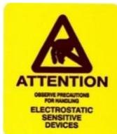
**THIS DEVICE IS ESD SENSITIVE.** OBSERVE PRECAUTIONS FOR HANDLING ELECTROSTATIC DISCHARGE SENSITIVE DEVICES IN ALL ASSEMBLY AND TEST AREAS (REF. JESD625).
