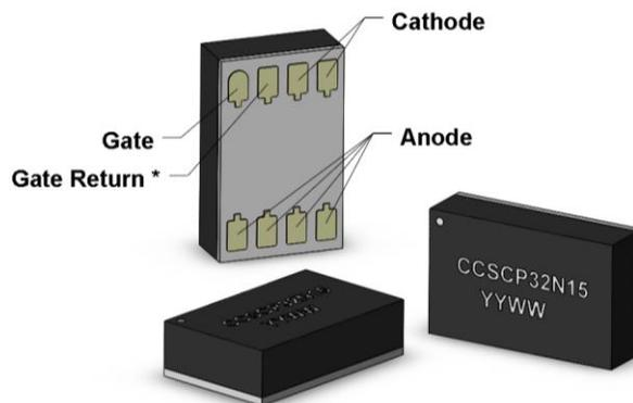
*\*The Gate Return pad provides a dedicated connection directly to the cathode of the semiconductor die. This connection consists of a single 0.010" aluminum bond wire.*
